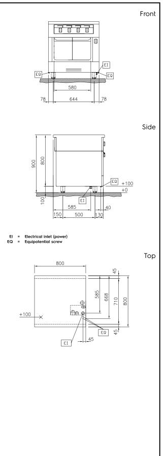
Electric Supply voltage: 588436 (MAIQFAH4AO) 400 V/3N ph/50/60 Hz 22 kW **Total Watts:** Key Information: On Oven; One-Side Configuration: Operated Front Plates Power: 5 - 5 kW **Back Plates Power:** 5 - 5 kW Front Plates dimensions: 320x330 320x330 **Back Plates dimensions:** 320x330 320x330 Induction Top Dimensions 800 mm (width): Induction Top Dimensions (depth): 800 mm External dimensions, Width: 800 mm External dimensions, Depth: 800 mm
